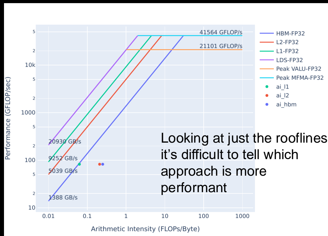
Solution FP32 Roofline
