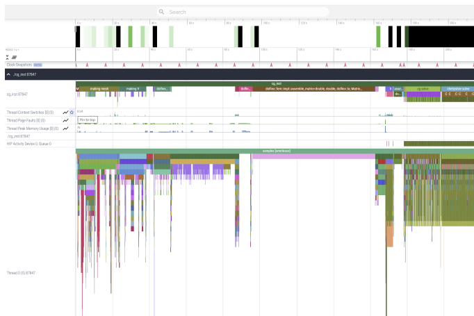
Figure: omnitrace profile of the whole application, 2 nodes, 8 GPU per node, 30m DoF per GPU. Profile from MPI rank 0
