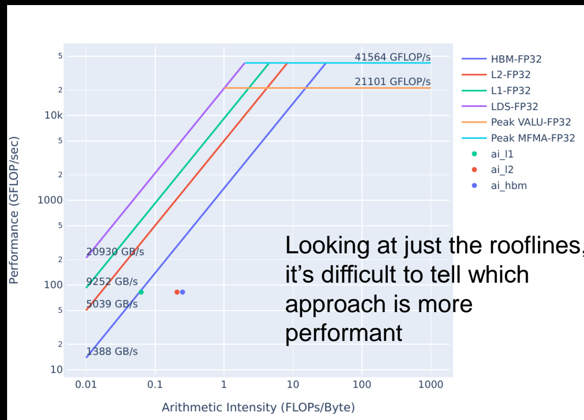
Solution FP32 Roofline
